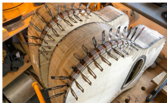
The sleek lines of Alex's bound arm bevel (far left) came to fruition with the help of a few dozen scalpel blades and copious amounts of supporting tape!
