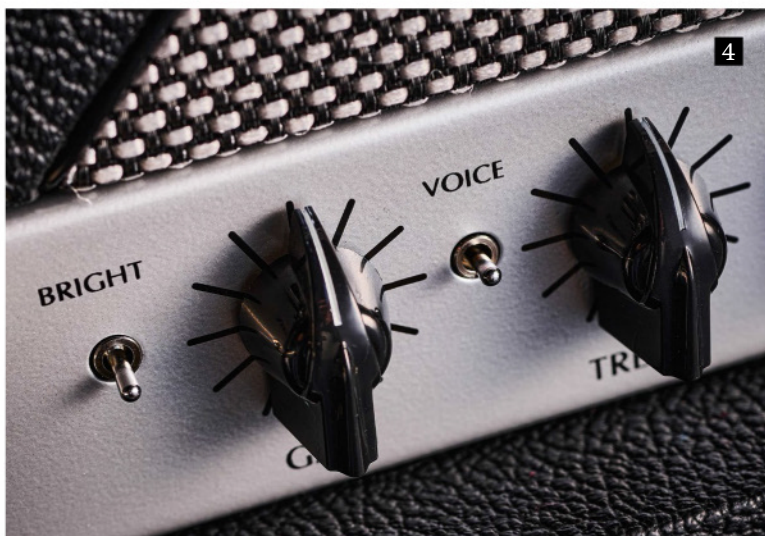
4. There are two three-way toggle switches: Bright gives two stages of treble emphasis plus an off; Voice adds around 6dB of gain, with an upper mid/treble boost, plus an off 5. The Deputy benefits from a simple fixed-level series effects loop. If you use time-based effects, like chorus or delay, this is the best place to plug them in to minimise noise and improve the effect depth
