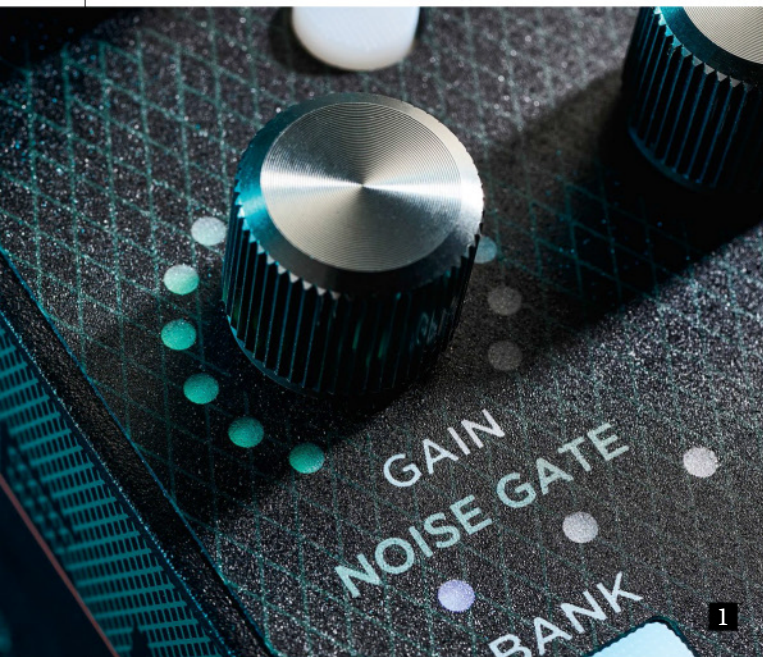
1. The Gain control is surrounded by a permanent ring of LEDs so you can instantly see how much gain is in use. Other controls make use of the bank/patch LEDs for a visual display
