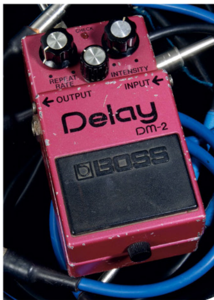
Boss's iconic DM-2 BBD analogue delay was released in 1981 as the compact pedal evolution of the larger-format DM-1 from 1978
