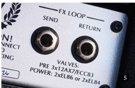
4. There are two three-way toggle switches: Bright gives two stages of treble emphasis plus an off; Voice adds around 6dB of gain, with an upper mid/treble boost, plus an off 5. The Deputy benefits from a simple fixed-level series effects loop. If you use time-based effects, like chorus or delay, this is the best place to plug them in to minimise noise and improve the effect depth
