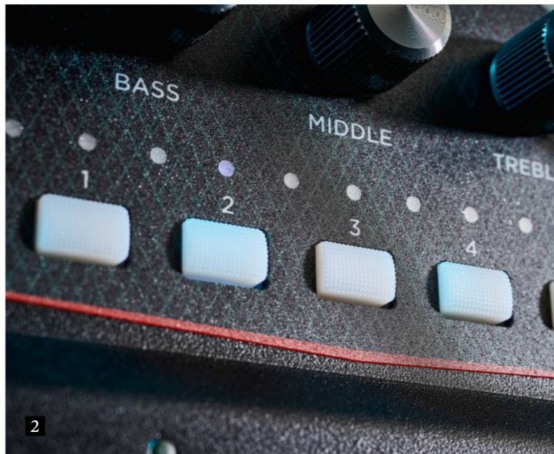
2. The Profiler Player can store up to 50 Rigs, organised in 10 banks of five, that are accessible from the footswitches or Bank select buttons. You can also get to these using Kemper's Rig Manager app, which works on desktops via USB or mobile devices via Wi-Fi
